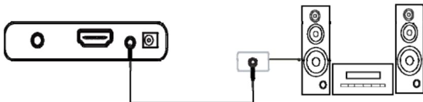
Coaxial output: Connect the Coaxial connector of the media player with the coaxial connector of other video or audio device by Coaxial cable. Then enter the product's audio output format interface, select the Digital Output option "RAW". It is available to enjoy 5.1 high quality sounds through a multi channel decoder/amplifier with coaxial input.
