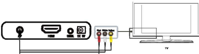
Plug the yellow connector into the AV output of product and AV input of TV, and plug the red and white
