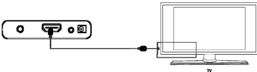
HDMI is an output with best audio and video effect which outputs digital video and audio composite at the same time. Connect HDMI cable to output of product and display device with HDMI input. Select HDMI mode in TV until it displays the interface of initiation.
